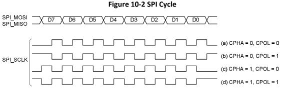
Figure 10-3 Different Clock Polarity/Phase
