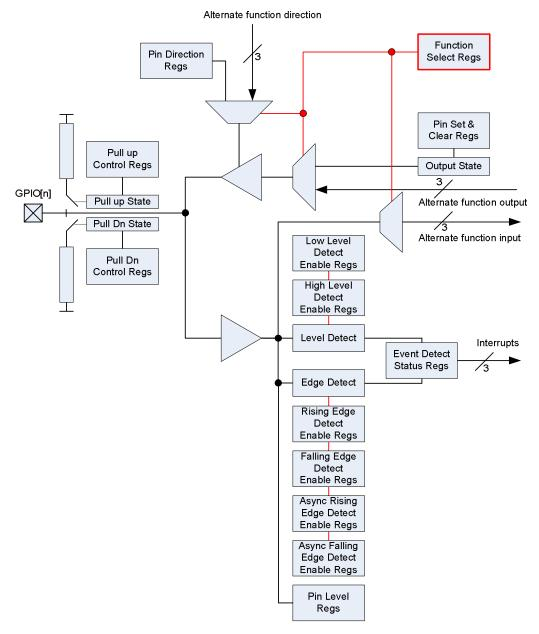
Figure 6-1 GPIO Block Diagram
