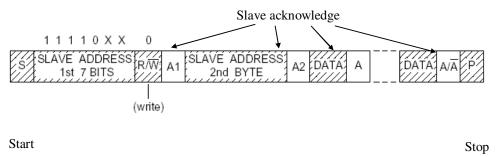
Figure 3-1 Write to a slave with 10 bit address
