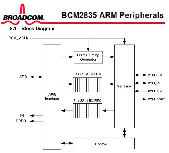
Figure 8-2 PCM Audio Interface Block Diagram
