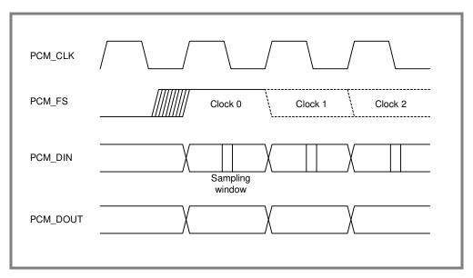
Figure 8-3 Timing at Start of Frame
