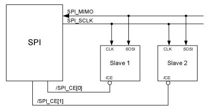
Figure 10-4 Bidirectional SPI Master Typical Usage
