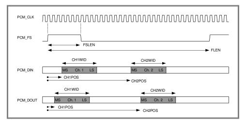
Figure 8-1 PCM Audio Interface Typical Timing
